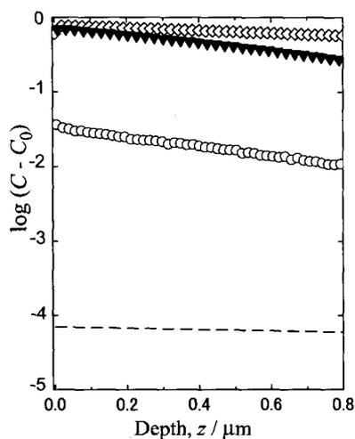
**Fig. 1** Depth profile of normalized relative concentration of  $^{18}\text{O}$  ( $C - C_0$ ) in YSZ single crystal annealed at  $T = 773\text{ K}$  for 300 s:  $\diamond$ ; sample A,  $\blacktriangledown$ ; sample B;  $\circ$ ; sample C. Dotted line is the calculated depth profile by eq. (5) with  $D_0^*$  and  $k$  data in dry  $\text{O}_2$  (1 atm = 1013 hPa) after Manning *et al.*<sup>5)</sup>
