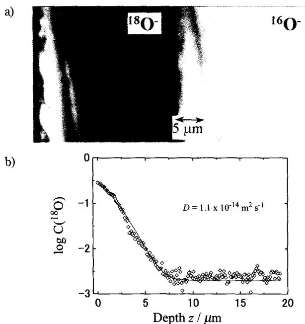
**Fig. 3** Concentration profiles of oxygen tracer on the cross section of sample B: (a) SIMS secondary ion images for  $^{18}\text{O}^-$  ion (left) and  $^{16}\text{O}^-$  ion (right). (b) line profile of relative concentration of  $^{18}\text{O}$ .
