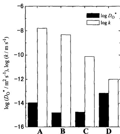
**Fig. 2** Oxygen tracer diffusion coefficient ( $D_0^*$ ) and surface reaction rate constant ( $k$ ) at  $T = 773\text{ K}$ : A, B, C corresponds to the data of sample A, B, C in table 2 respectively. D; literature data obtained in dry  $\text{O}_2$ .<sup>5)</sup>
