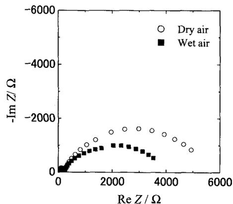
Fig. 4 Effect of atmospheres on complex impedance plots for YSZ polycrystalline with platinum electrodes at  $T = 761$  K: □; dry air ( $100 \text{ ml min}^{-1}$ ) for both sides of YSZ, ■ cathode side: air +  $H_2O$  (7.6 hPa), anode side: dry air.
