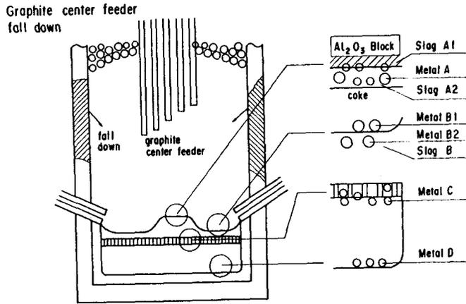
Fig. 2 Schematic dissection diagram of AR-3: A part of furnace walls fell down and the graphite center feeder was burnt at the tip.
