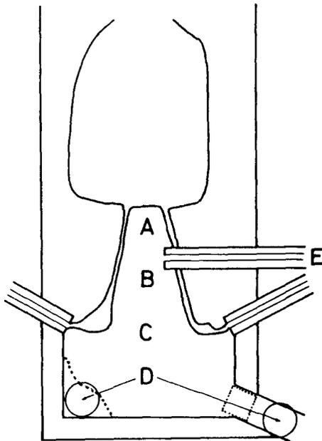
Fig. 3 Schematic dissection diagram of AR-4: Oxygen migrated path was formed in the accumulated products. For compositions of samples at A - D, see Table 2.
