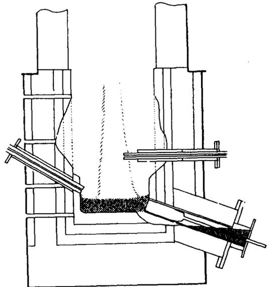
Fig. 4 Schematic dissection diagram of AR-14: The wall alumina was melted and the products flowed into the hearth and tap hole. There was no gas stream inside a cone formed at the center of furnace.
