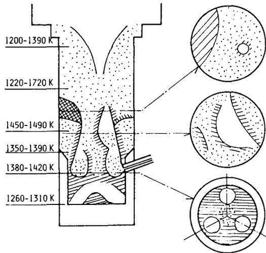
Fig.2 Dissection diagram of BR-4 with wall temperatures:
