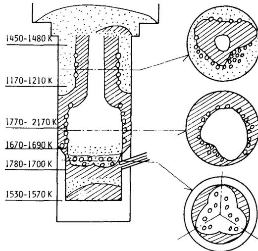
Fig.3 Dissection diagram of BR-8 with wall temperatures:
